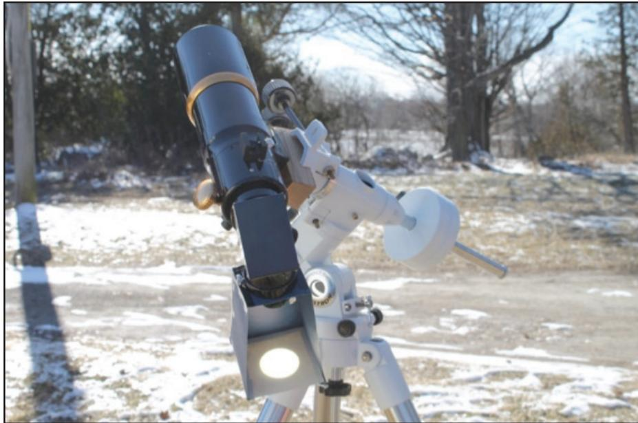
*Eyepiece projection through a refractor using a Hossfield pyramid.*
